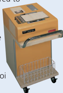
In 1979, Fukuda Denshi began sales of the FCP-30, Japan's first ECG with an onboard computer for automated analysis.
