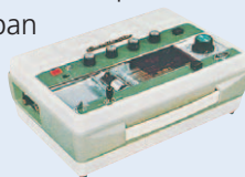
The RS-102T, a fully transistorized hot-pen direct-recording ECG, went on sale in 1968.
