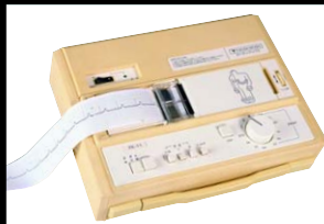
Isolation Amp adopted ECG FK-11 Since 1982, the Isolation amp has assured a high level of safety for patients
