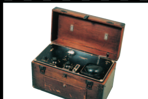
Vacuum-tube, Battery-operated, Photographic one-channel ECG First ECG in Japan
