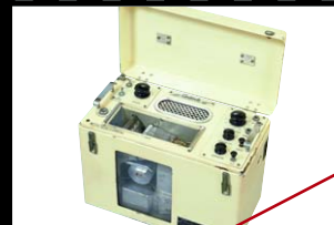
Heat Pen • Direct Writing ECG RS-1 Produced from 1951, Differential Amp adopted, First direct-writing ECG.
