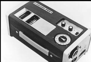
All-transistorized ECG FCC-1 Produced from 1968, Heat pen writing, All-transistorized, one-channel ECG
