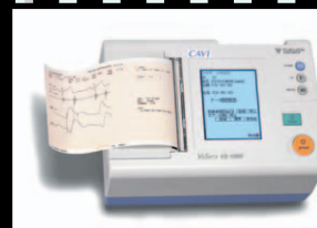
Vascular Screening VS-1000 CAVI Diagnostic equipment for measuring blood pressure and pulse waves
